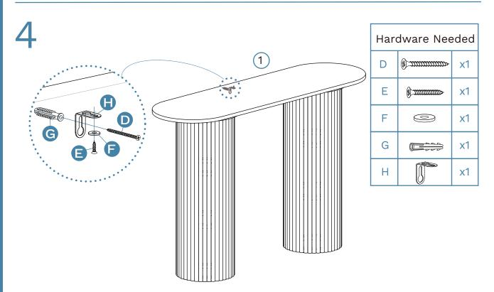
Once assembled lift furniture into place, do not drag. Attach connection plate to the top panel with 1x washer (F) and 1x screw (E). Use a drill to create a small hole lining up with the connection plate (H). Fasten to wall using 1x wall anchor (G), 1x wall screw (D). Ensure unit is balanced and steady before use. You're done, enjoy!
